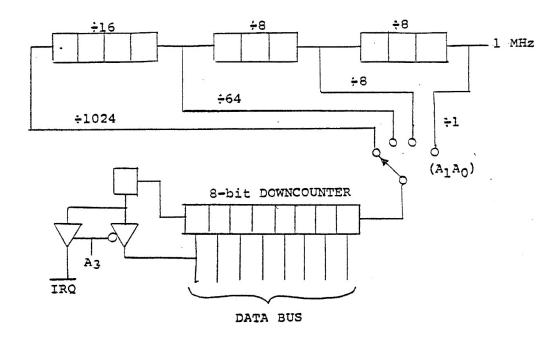
The clock which drives the downcounter is one of four selected rates. The fastest rate is the microprocessor's 1 MHz crystal clock. This clock is also applied to a tapped binary dividing chain, giving clock periods of 1, 8, 64, and 1024 microseconds. The last, and slowest clock is about one milliseconds, giving a maximum timable delay of about one quarter second.
