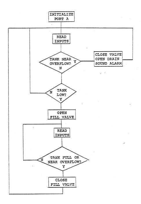
2. Assemble the program which follows. You will have to calculate the relative offsets for two of the branch instructions. Note that in the main loop of the program the input information is loaded and rotated right twice. The figure below shows the results of these operations.
